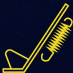
SIDE STAND INDICATION AND ENGINE CUT-OFF
